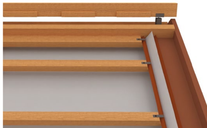
Fixing of finishing trim by staples
